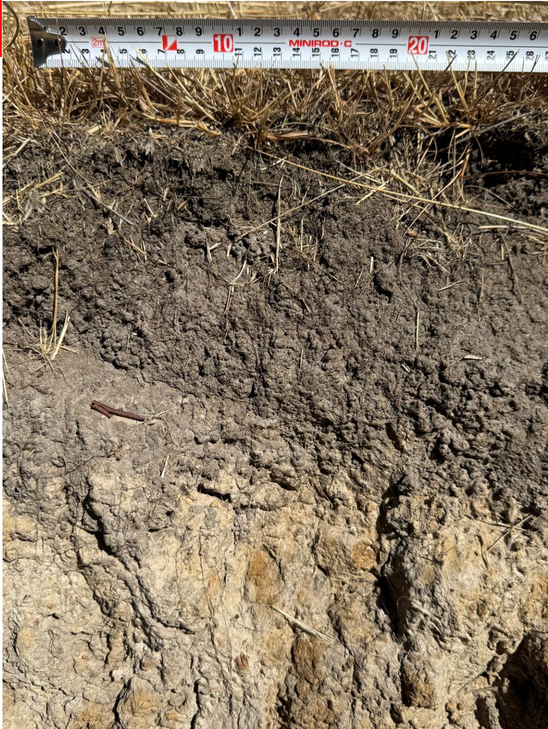
Image 14 Texture contrast soil, with a sandy loam topsoil over a yellow/brown clay subsoil which covers the majority of the subject property. (Taken on site visit 20/2/26).
