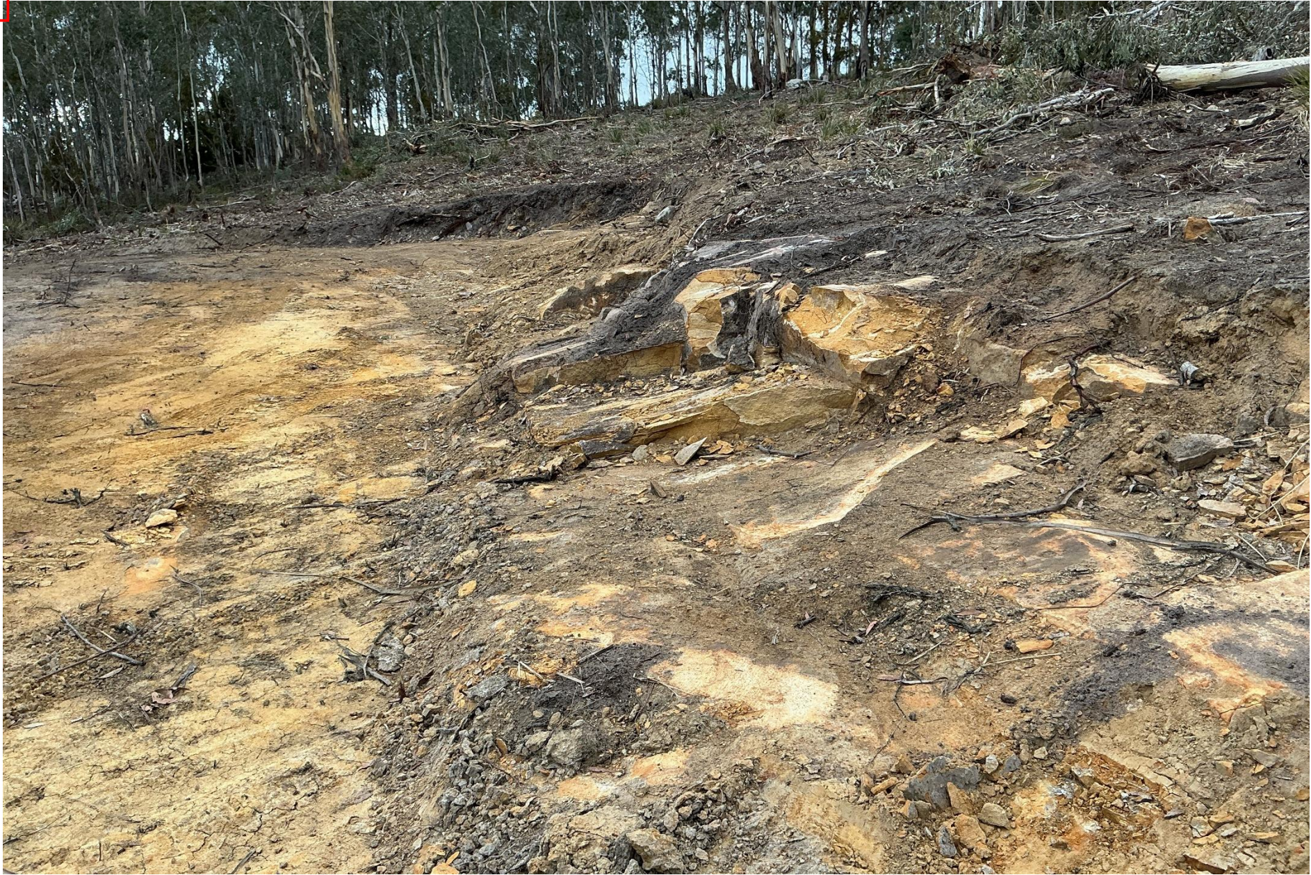
Photo 2 Showing the proposed shed location with exposed sandstone bedrock
