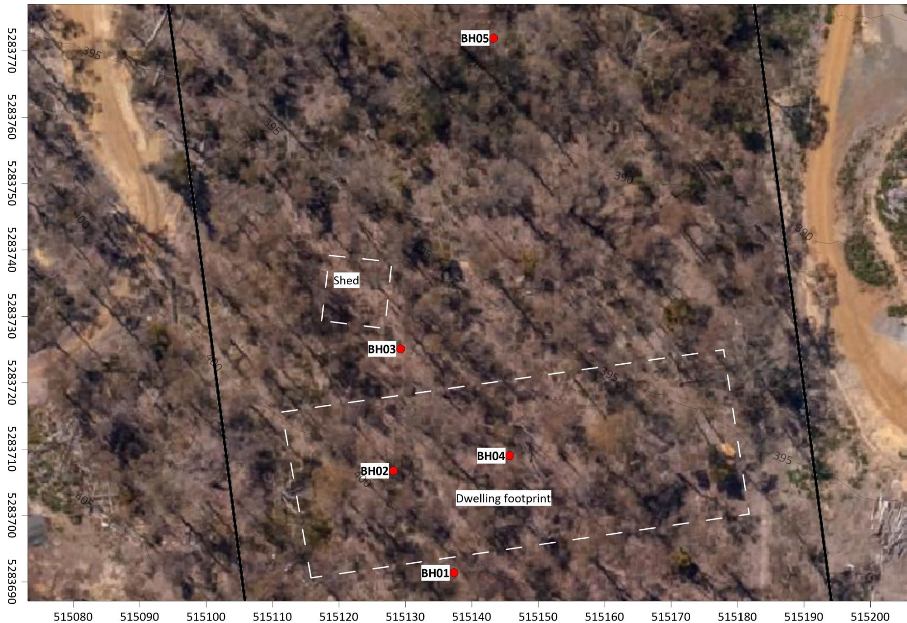
Figure 1 Site Borehole Locations
