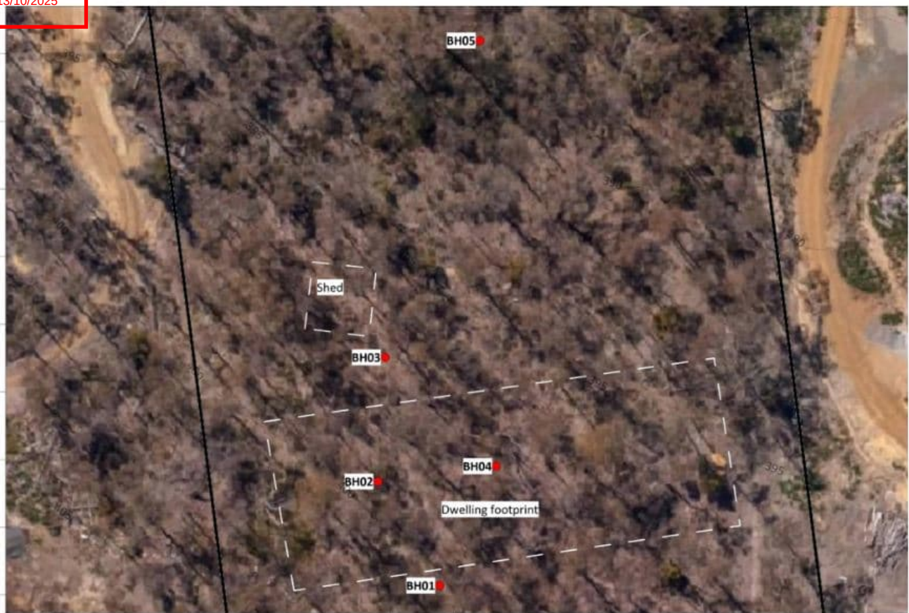
Figure 3 – Bore Hole Test Location
