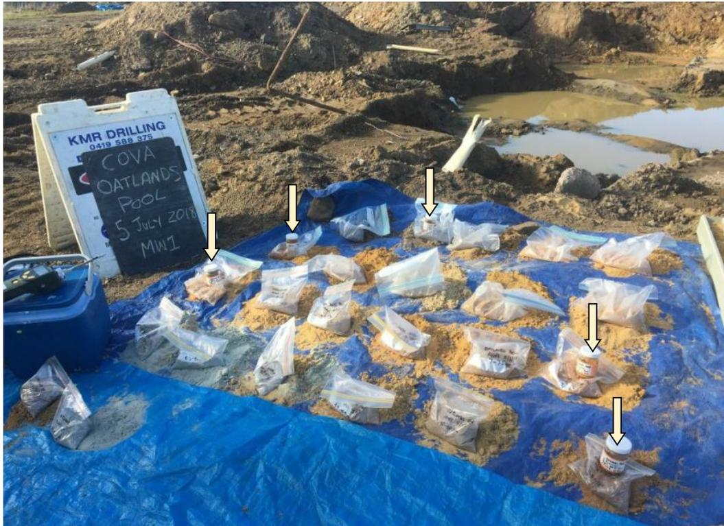
Plate 1.3 (above). Continuous drill-return samples (sand) bagged at 0.5m intervals. These were tested on site (and 24 hours later in the office) with a PID. Five samples (arrowed) were collected for laboratory analysis for petroleum hydrocarbons. Start is at top left; end is at bottom right.
