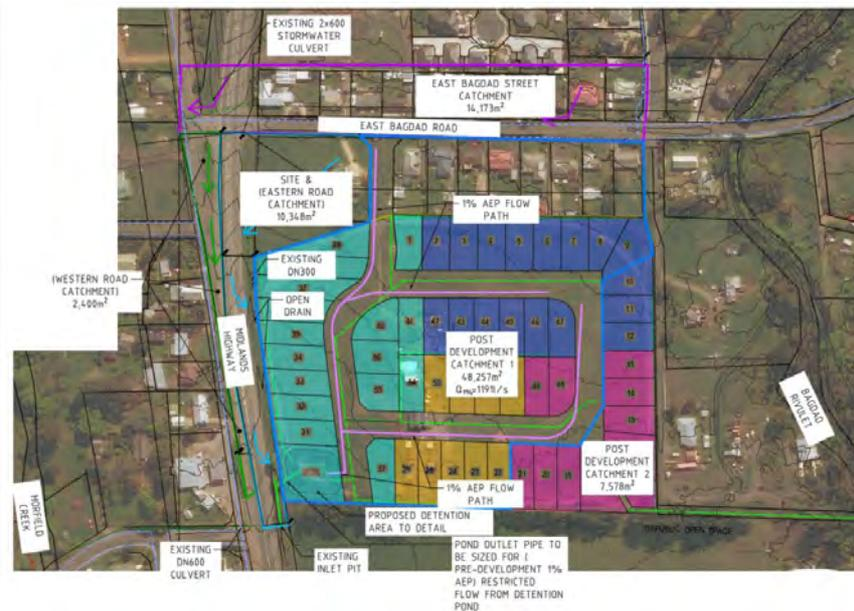
Image 8 - Proposed Stormwater Catchments
