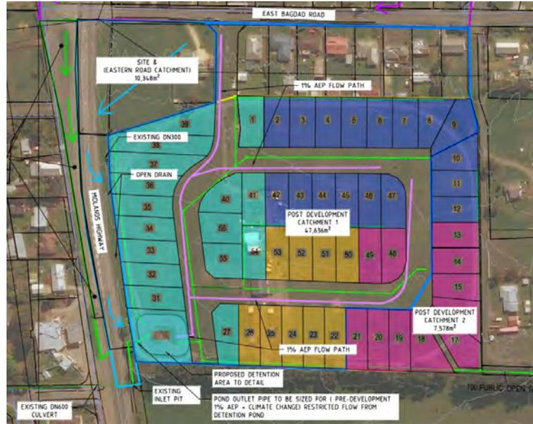
Image 3 - Proposed Stormwater Catchments
