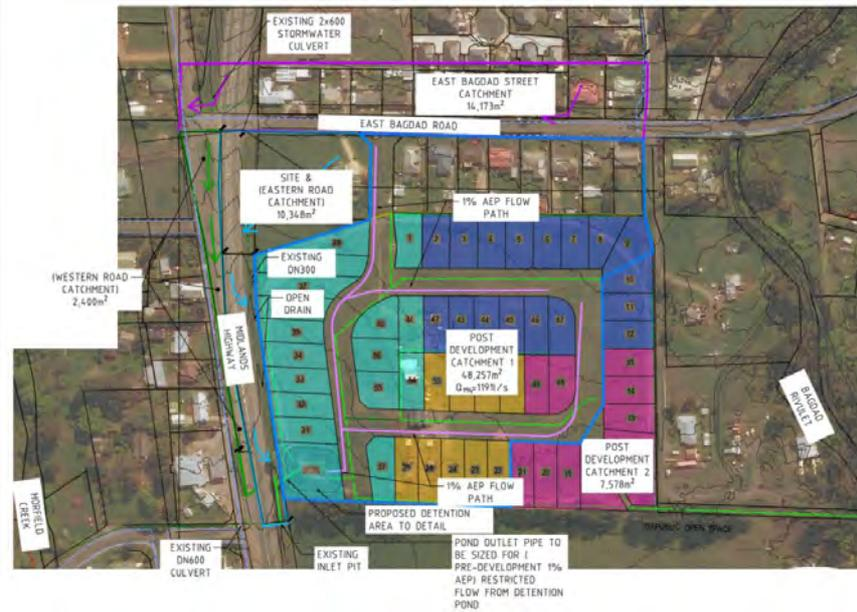
Image 8 - Proposed Stormwater Catchments
