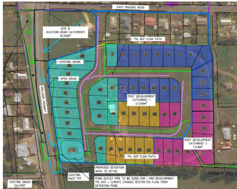
Image 3 - Proposed Stormwater Catchments
