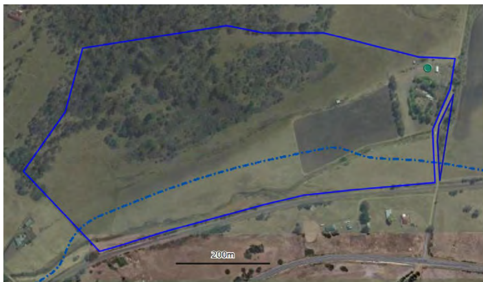
Figure 16 Tas Irrigation “Main Line 2” pipeline (blue dotted line) crossing the southern area of the property (outlined in blue) and the location of the proposed cool storage facility (green dot)
