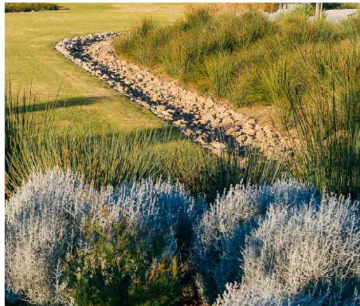
Directing stormwater off roads and other hard surfaces into the WSUD gardens can help filter pollutants as well as watering the plants.
